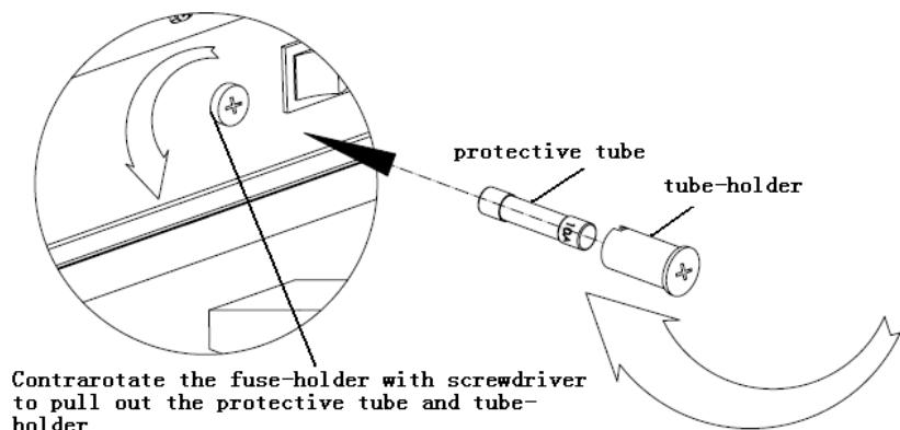
Contrarotate the fuse-holder with screwdriver
